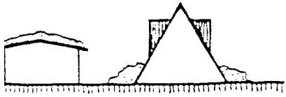
Flat or Shallow Pitched Roofs Hold Snow for Added Insulation
